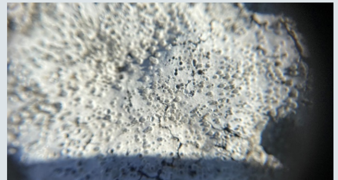
Solvent acrylic bead coverage
